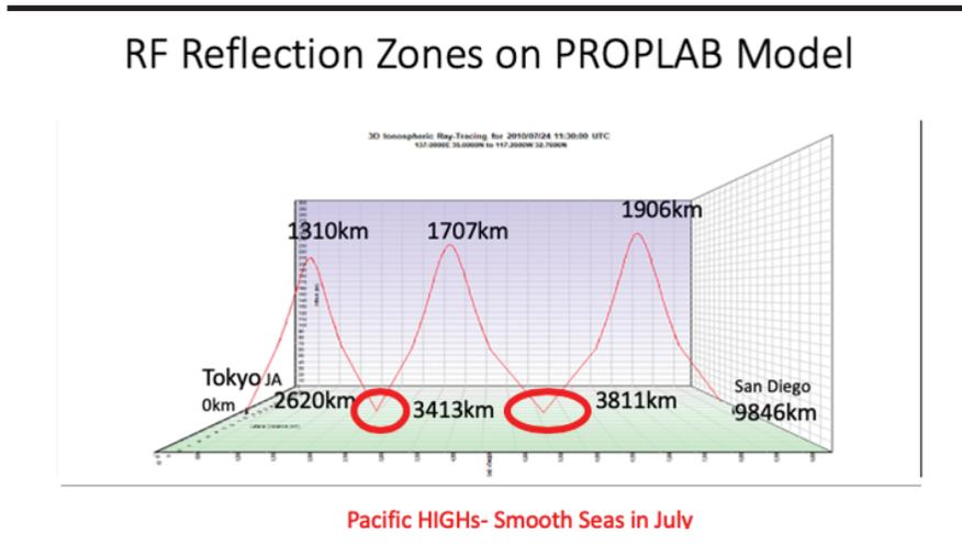
Figure 1 — PROPLAB 3-hop Tokyo – San Diego model for July 24, 2010, with superimposed data.
