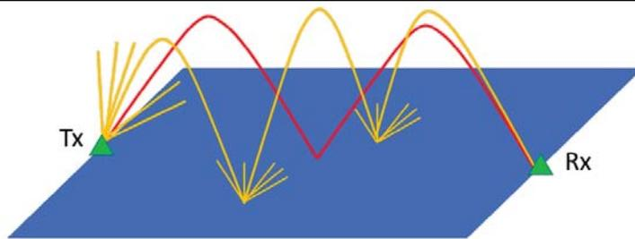
Figure 3 — Illustration of multiple diffuse scattered waves on a 2-hop model.
