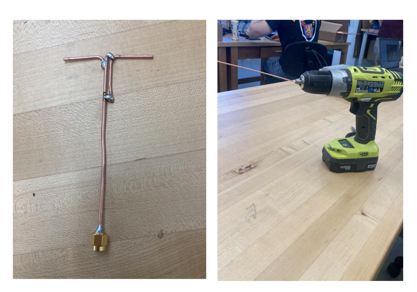
Fig. 1: A) Completed dipole antenna with superb soldering job. B) Steve Cerwin's pro-tip to straightening and strengthening copper.
