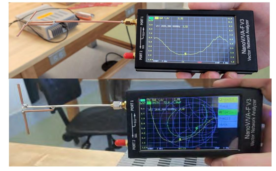
Fig. 2: Matthew Dittmar's dipole antenna being tested using a NanoVNA.
