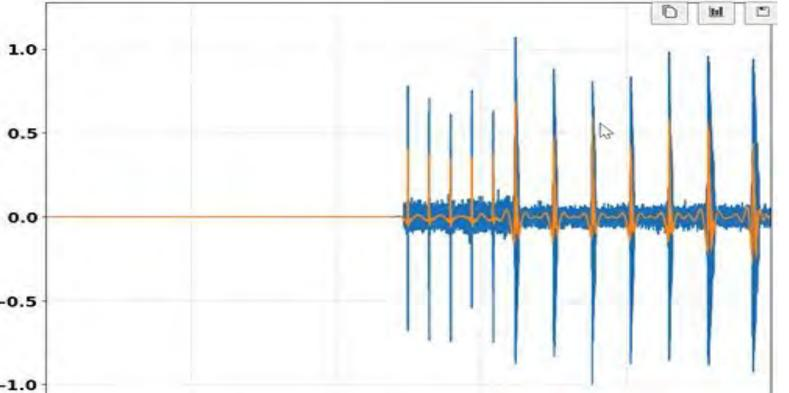
Fig. 2 The correlated result from the given tx3.wav file that enables us to find the starting point of each chirp
