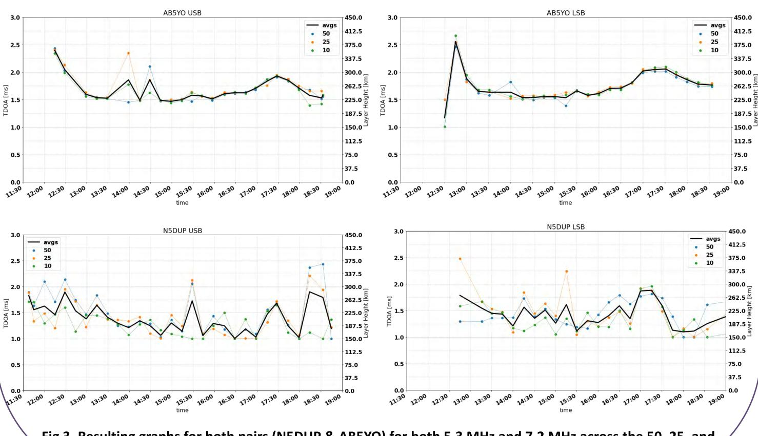
Fig 3. Resulting graphs for both pairs (N5DUP & AB5YO) for both 5.3 MHz and 7.2 MHz across the 50, 25, and 10 Hz/ms sweep rates
