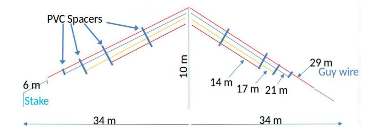
Figure 1. Antenna setup
